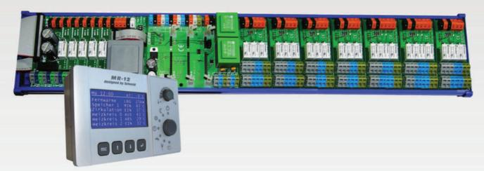
Universally useable, modulary structured heating regulator with basis on a freely programmable micro-controller with extensive possibilities for Bus-Connections, system display, remote maintenance and web-connection.
